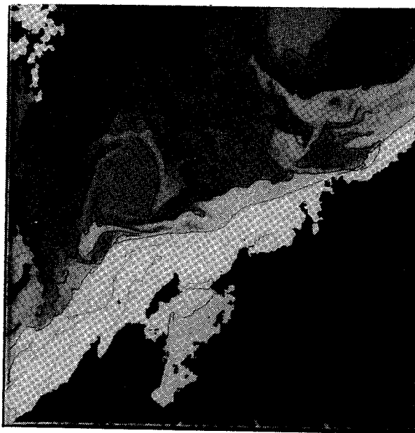
Figure 5: SST fields off Cape Hatteras with clouds zeroed out and edges overlaid (thin black lines).
