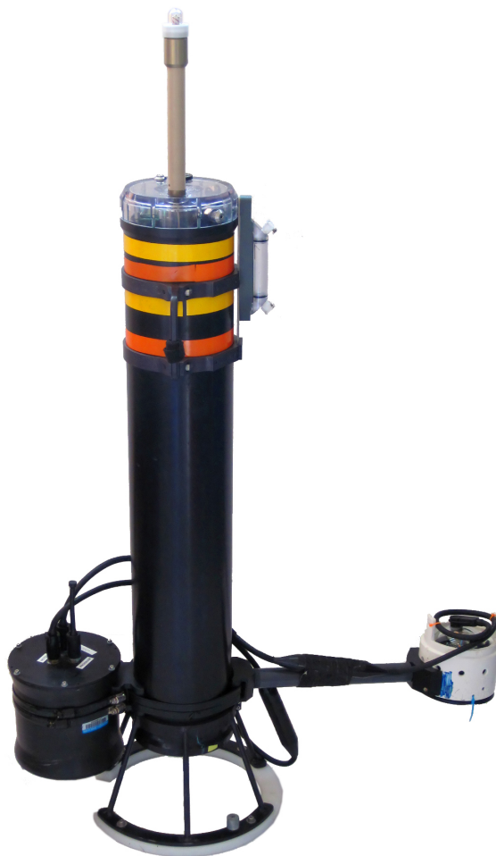
Figure 1. Lagrangian Float with Cameras and Strobe
