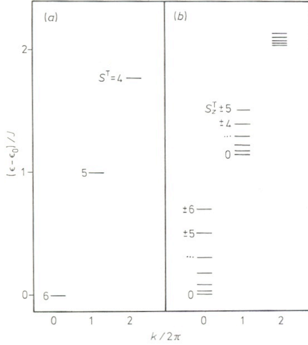
Figure 2. (a) Lowest energy levels of the isotropic s = 1 Heisenberg ferromagnet consisting of six spins. The states shown belong to the three categories mentioned in the text. (b) Lowest multiplets of eigenstates for the planar s = 1 Heisenberg ferromagnet, into which the states in (a) split, when the anisotropy is switched on.
