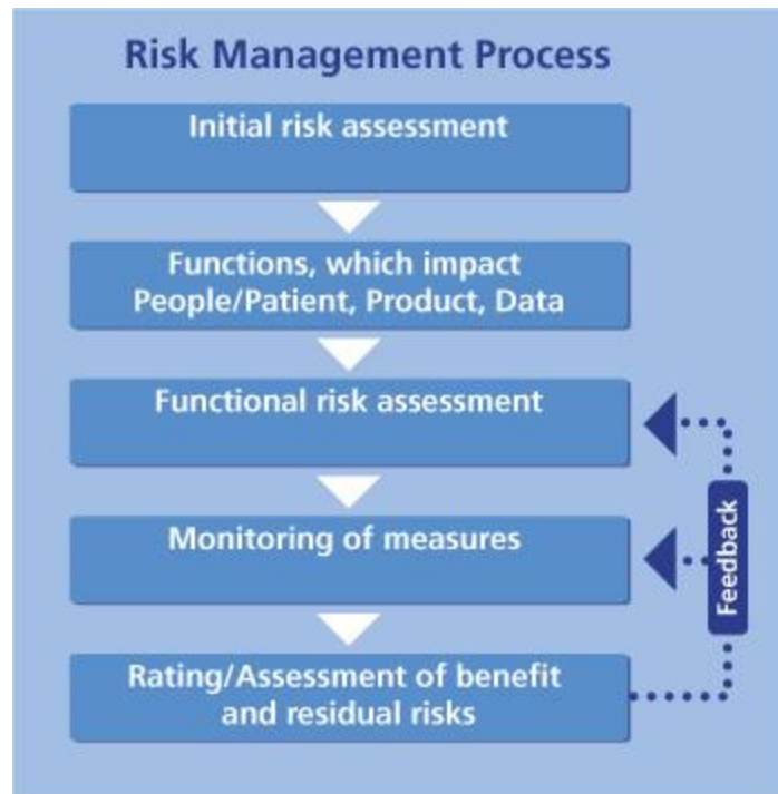
Figure 29: Five ‘Risk Management Process’ steps [Source: 19] shows how the risk assessment is performed to determine the extent of validation testing required.
