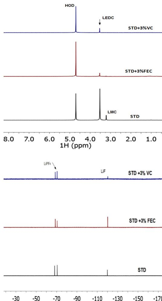
**Figure 8.** (Top)  $^1\text{H}$  NMR spectra of the  $\text{D}_2\text{O}$  extracts of BF-graphite electrodes cycled with three different electrolytes, 1.2 M  $\text{LiPF}_6/\text{EC}:\text{EMC}$  with 3% VC, 1.2 M  $\text{LiPF}_6/\text{EC}:\text{EMC}$  with 3% FEC, and 1.2 M  $\text{LiPF}_6/\text{EC}:\text{EMC}$  (STD). (Bottom).  $^{19}\text{F}$  NMR spectra of the  $\text{D}_2\text{O}$  extracts of BF-graphite electrodes cycled three different electrolytes.
