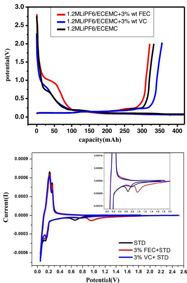
**Figure 1.** (Top) potential vs. capacity curves for BF-graphite/Li cells with 1.2 M LiPF<sub>6</sub>/EC:EMC 3:7 v/v (STD), STD with 3 wt% VC and STD with 3 wt% FEC. (bottom) cyclic voltammetry, scan rate of 0.5 mV/s, for the three different electrolytes with in BF-graphite/Li coin cells.
