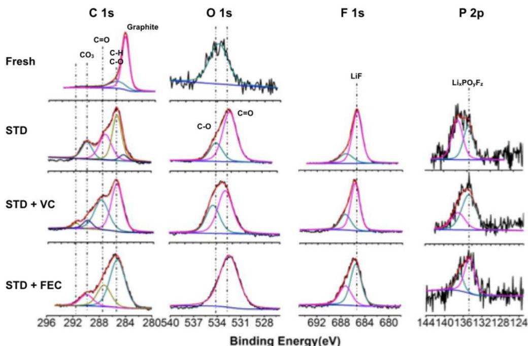
**Figure 2.** C 1s, O 1s, F 1s, and P 2p XPS core spectra of BF-graphite electrodes after the first cycle with 1.2 M LiPF<sub>6</sub>/EC:EMC (30:70 v/v) as the standard electrolyte (STD), STD with 3% FEC and STD with 3% VC.
