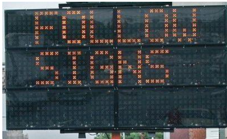
Figure 1. Variable Message Sign (VMS) with 50 x 24 Pixilated Board
