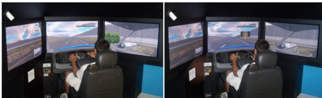
Figure 10. Driving Simulator Views, left: Driver approaches marker, right: VMS message in view
