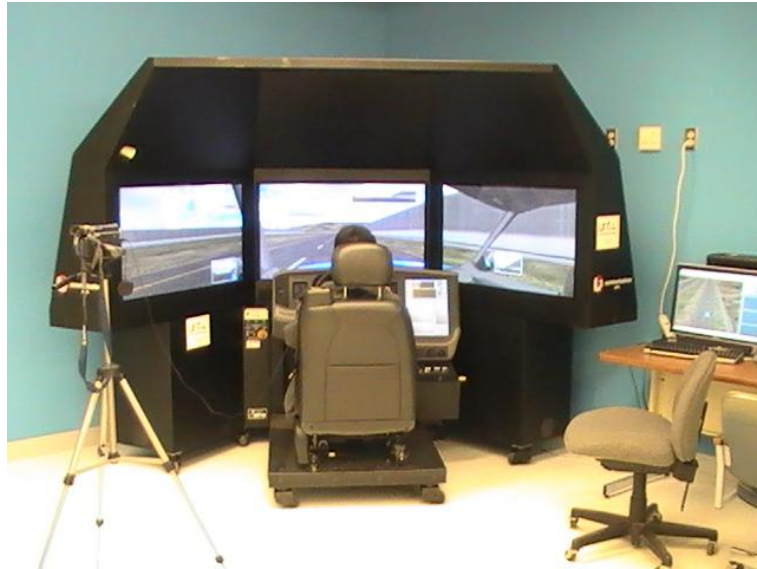
Figure 13. Driving Simulation Experiment Setup in Driving Performance Lab at URI
