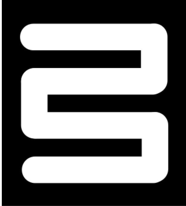
Figure 9: Example of a microfluidic channel designed in Inkscape; the printer prints the black areas, whereas the channels are left blank
