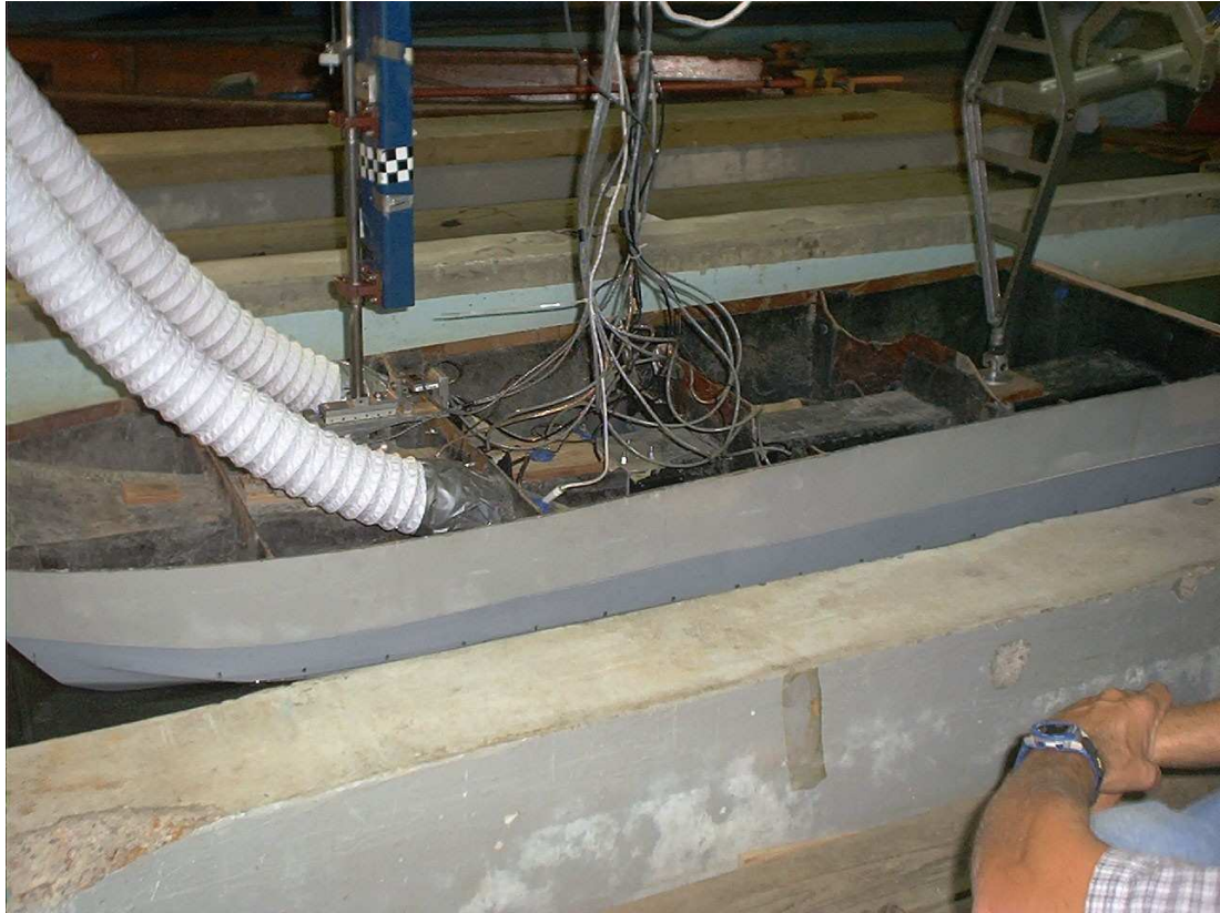
Figure A.19. Side view of model setup used in early tests not considered in manuscript, where air cushion ducting was attached from the bow. Note tow mount (left), instrument cabling (center), and grasshopper (right).
