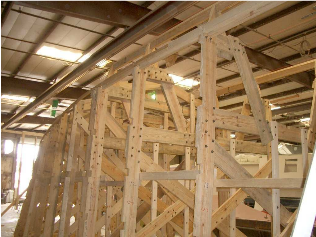
Figure A.24. Close-up of part of the wooden frame (i.e., plug) for a demihull of the Gladius .
