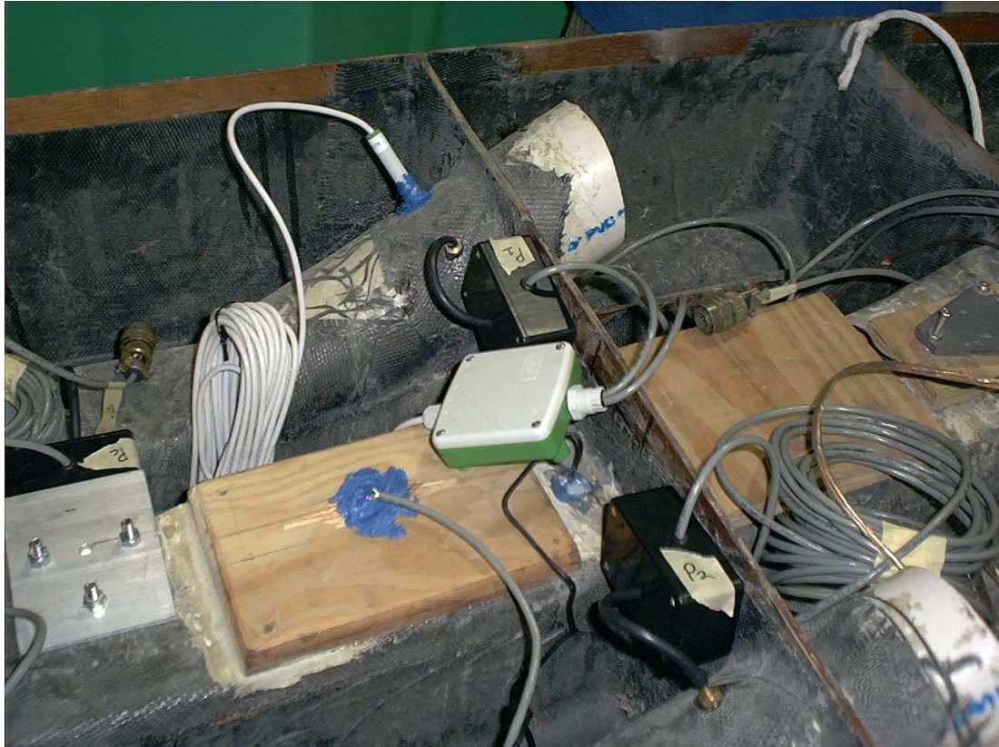
Figure A.7. View of the sensors used at the bow, including a hot film anemometer attached to the port air cushion inlet, and pressure sensors P_1 , P_2 , and P_c . Note the plate used for attaching the tow mount (right).
