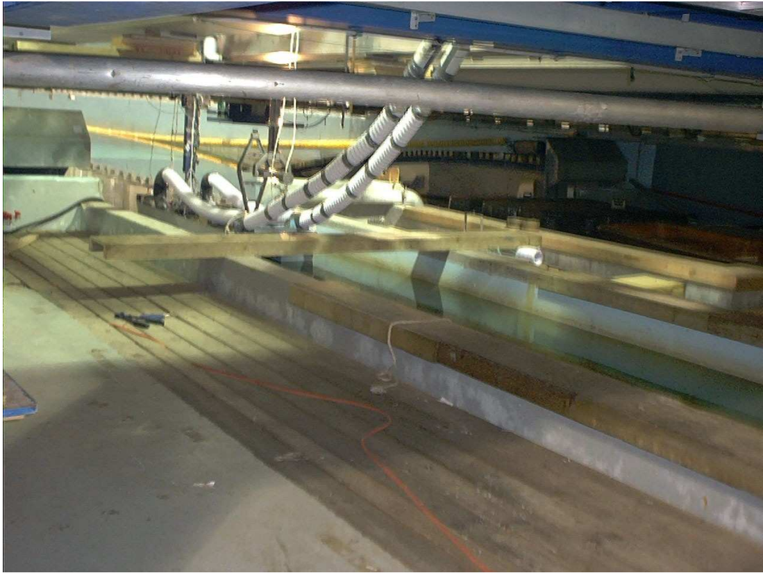
Figure A.11. 2.3 m model in position underneath the tow carriage. Note the ducting between the blower (not seen) and the air cushions.
