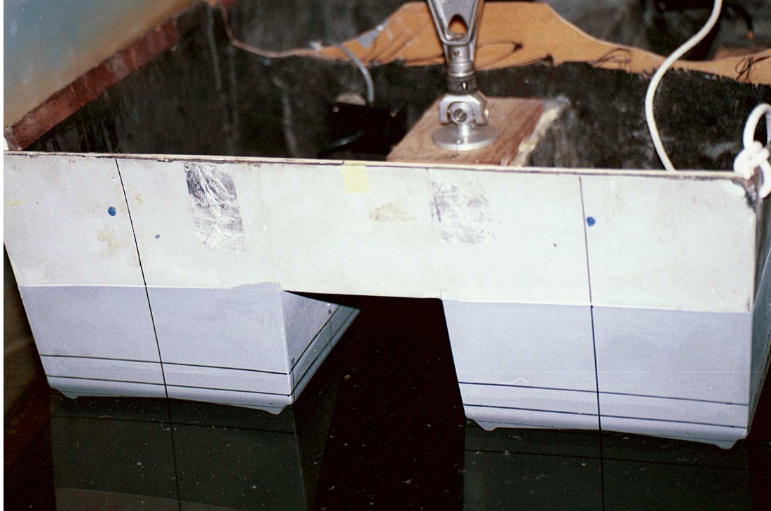
Figure A.4. Stern view of the 2.3 m model, with lines marking draft. Note the grasshopper attachment amidships, and the cord attached in the corners to help pick up the model for adjustments.
