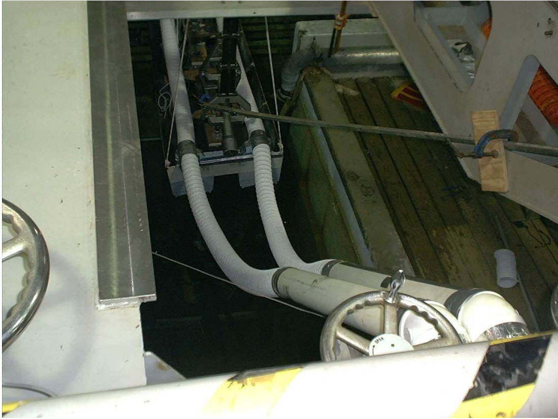
Figure A.15. Top view of model from tow carriage, showing how the ducting reaches between the blower (not seen, bottom right), and the model (top left).
