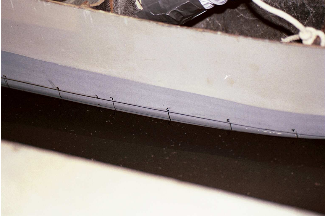
Figure A.5. Close-up of the starboard bow of the 2.3 m model, with lines marking draft, and numbering indicating distance from the bow. Note the ducting attached (top) and the cord attached in the corner to help pick up the model for adjustments (top right).
