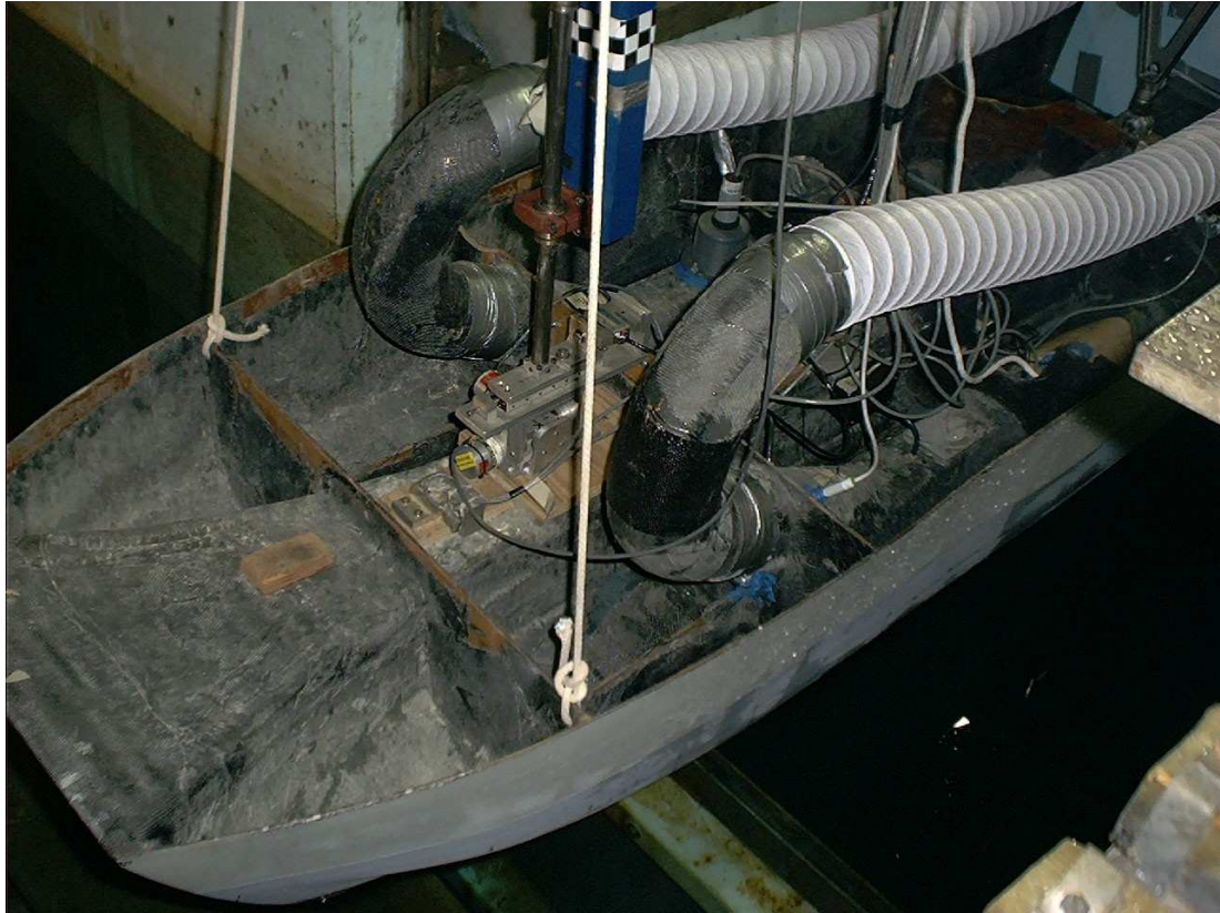
Figure A.12. Front view of the 2.3 m model, with tow mount, air cushion ducting, pressure sensors, and range finder attached. Note the model is being held out of the water by cord attached to the four corners of the model.
