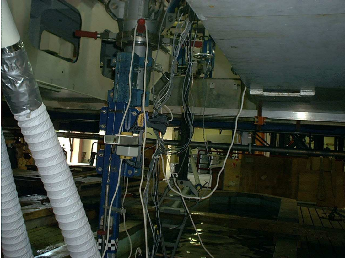
Figure A.18. Close up of tow mount and instrument cabling between model and tow carriage.
