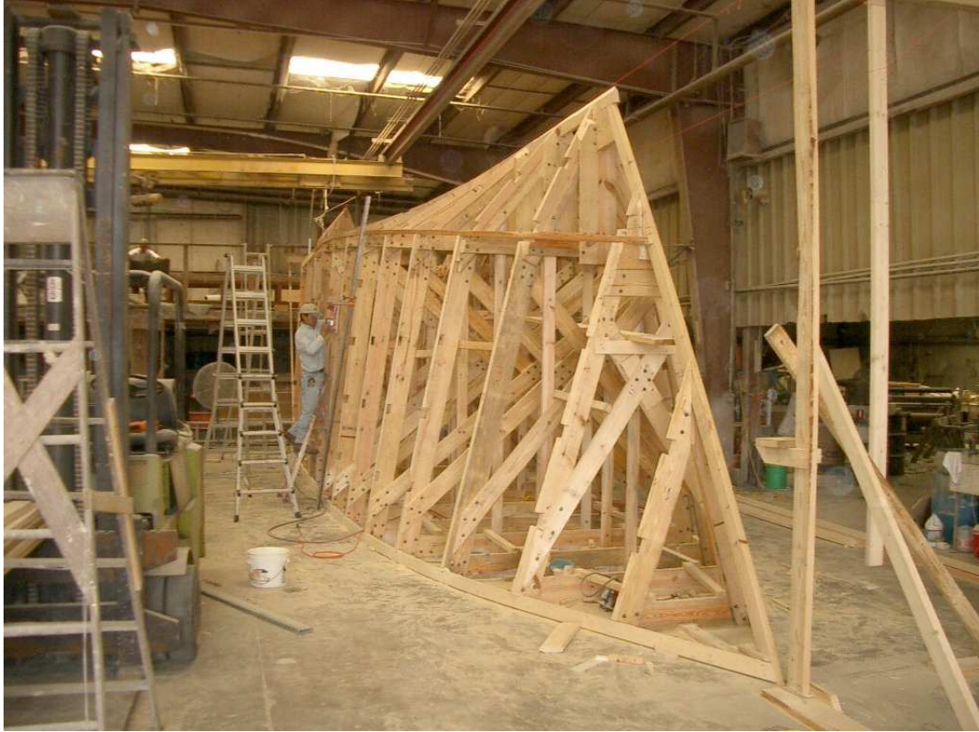
Figure A.20. Fore end of the wooden frame (i.e., plug) for building a demihull of the Gladius .
