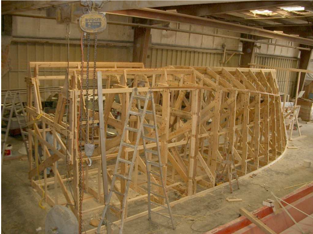
Figure A.22. Fore end of the wooden frame (i.e., plug) for a demihull of the Gladius .
