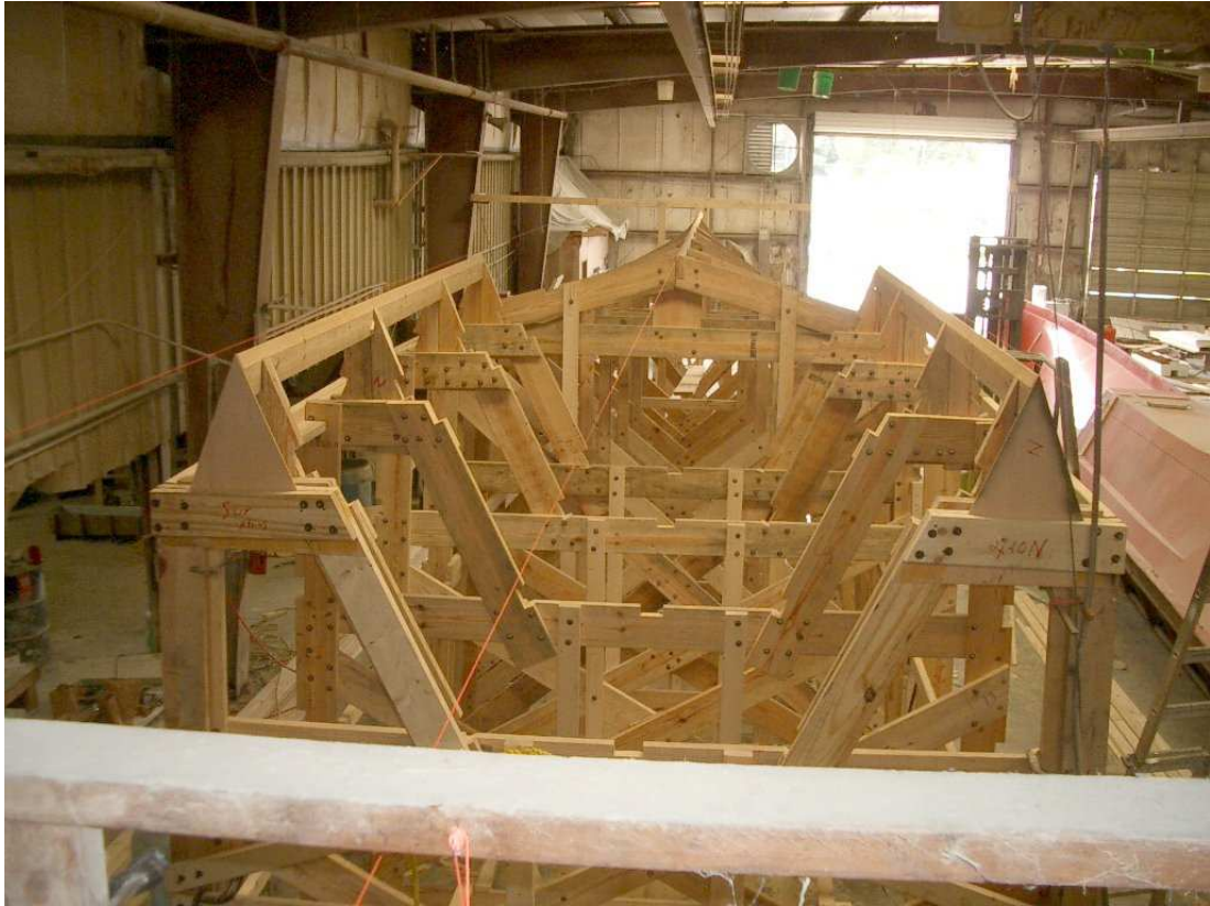
Figure A.23. Fore end of the wooden frame (i.e., plug) for a demihull of the Gladius (foreground), and resulting mold (right background).
