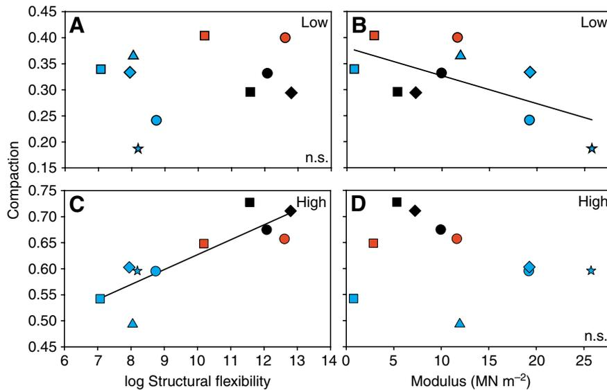
Fig. 5. Compaction, the proportion of area lost because of reconfiguration, versus structural properties. (A,B) Low velocity ( $0.5 \text{ m s}^{-1}$ ). (C,D) High velocity ( $3.0 \text{ m s}^{-1}$ ). Regression of low velocity compaction to modulus (slope= $-0.005$ ,  $R^2=0.39$ ,  $P=0.05$ ) and high velocity compaction to log structural flexibility were significant (slope= $0.029$ ,  $R^2=0.73$ ,  $P<0.01$ ). Other regressions were not significant ( $P>0.05$ ). Species labeled as per Fig. 4.
