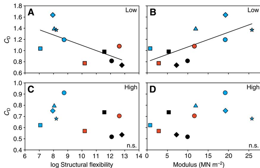
Fig. 6. Drag coefficient versus structural properties. (A,B) Low velocity ( $0.5 \text{ m s}^{-1}$ ). (C,D) High velocity ( $3.0 \text{ m s}^{-1}$ ). Linear regressions of  $C_D$  to log-transformed structural flexibility (slope= $-0.093$ ,  $R^2=0.47$ ,  $P=0.03$ ) and  $C_D$  to modulus (slope= $0.026$ ,  $R^2=0.50$ ,  $P=0.02$ ) were significant at low velocity. Neither relationship was significant at high velocity ( $P>0.05$ ). Species labeled as per Fig. 4.
