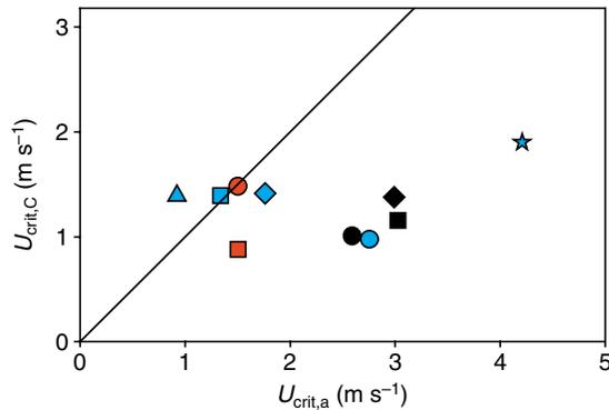
Fig. 7. The critical velocities of normalized area ( $U_{crit,a}$ ), the velocity at which area reaches within 5% of the minimum area, versus the critical velocity of drag coefficient ( $U_{crit,C}$ ), the velocity at which  $C_D$  reaches within 5% of the minimum  $C_D$ . The line is unity. Note that most species fall below the line, indicating that  $C_D$  asymptotes at a lower velocity than normalized area for those species. Species labeled as per Fig. 4.
