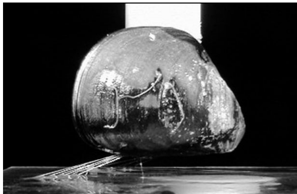
Fig. 2. One valve of each mussel was fixed to a vertical nylon rod using cyanoacrylate glue, which was then suspended 6.5 mm above an acrylic plate. During each experiment, mussels gradually tethered themselves to the acrylic plate by producing byssal threads.
