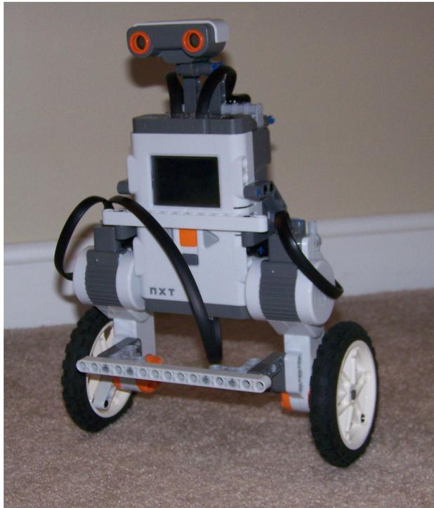
Figure 4.1. LEGO Two-wheeled Robot
