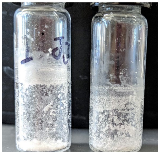
Figure 2: Examples of cyclodextrin-MOF solids made by two different students, after a 7-day crystallization period, followed by multiple washes with dichloromethane and oven drying of the samples
