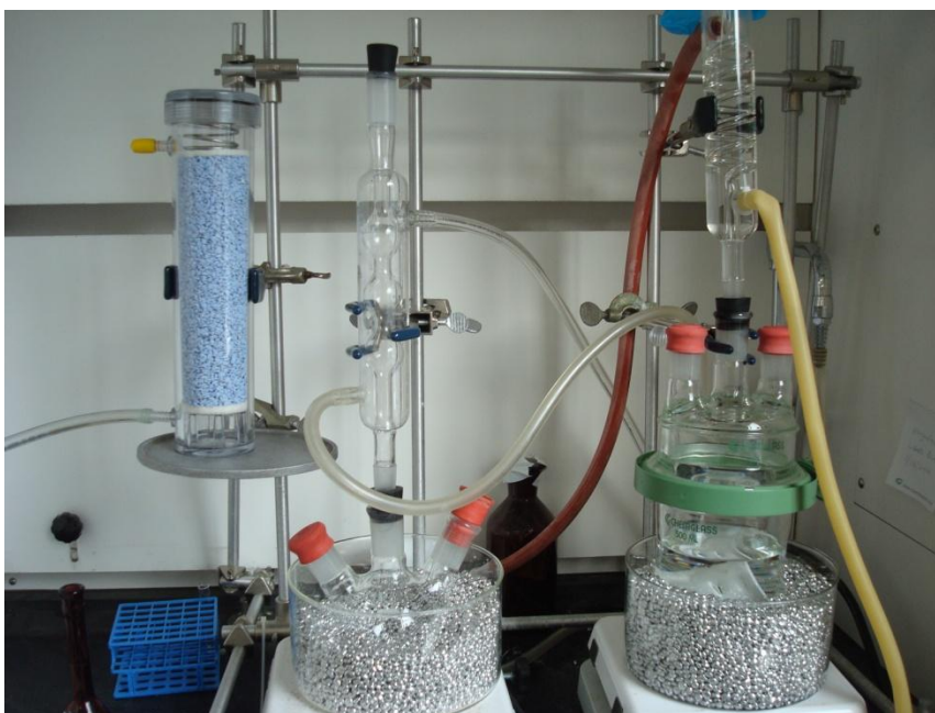
Figure 3.3: Experimental setup of the PS, PAA, and PS- b -PAA modification of glass substrate via ATRP.
