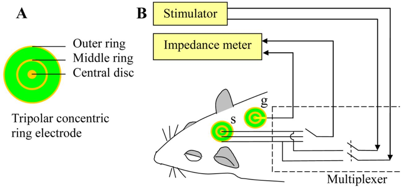
**Fig. 1.** Schematic representations of the tripolar concentric ring electrode (A) and the experimental setup (B). The TFS was applied between the outer ring and the central disc of electrode (s). Electrode (g) was the ground.
