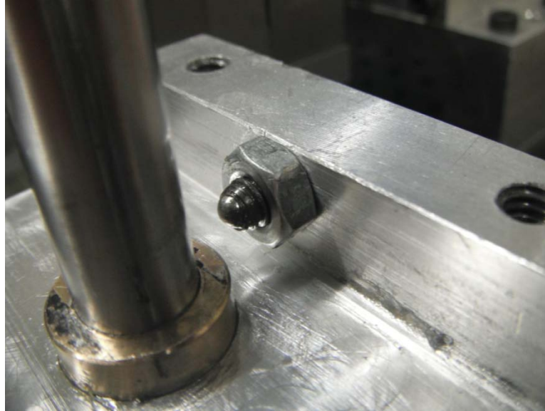
Figure 5. Photograph of the ball bearing set screw shown mounted in the support tower. Before testing begins the screw is tightened against the face of the specimen and the nut is tightened to resist loosening due to vibration.
