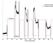
**Fig. 5.** Real-time performance of the designed NMI system. The decision stream (0: sitting, 1: standing) is aligned with the pressure data (black solid line) measured under the gluteal region of the subject.
