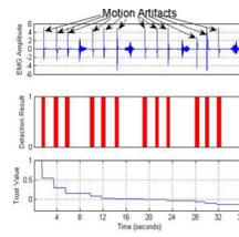
**Fig. 7.** Real time performance demonstration of the abnormal detector under motion artifacts. The representative EMG signals(upper panel), the detection results of CUSUM (middle panel), and the trust value (lower panel) are demonstrated
