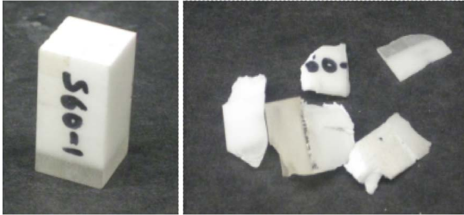
Figure 44. Impacted specimen of S60-040-5FGM
