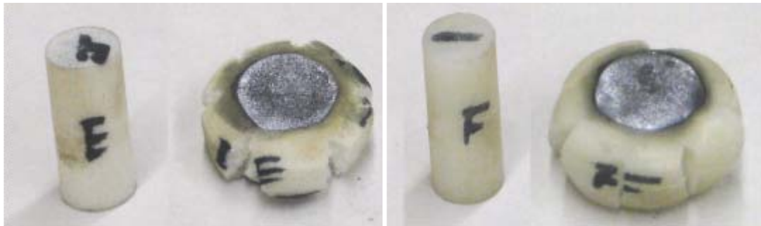
Figure 32. Cracks formation on K1-40 (left) and K1-10 (right) type syntactic foams
