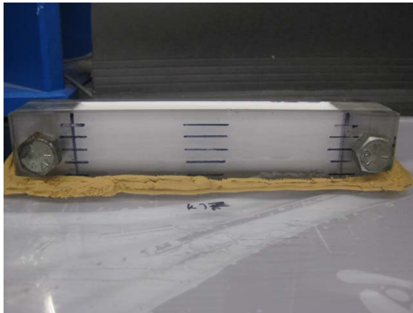
Figure 1. Casting Mold for Preparation of FGMs
