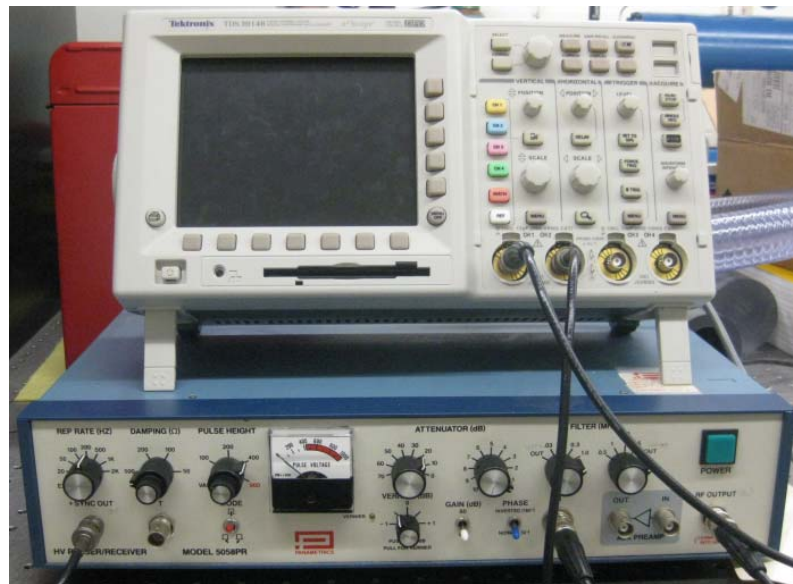
Figure 10. Cable connection of Pulser/Receiver and oscilloscope
