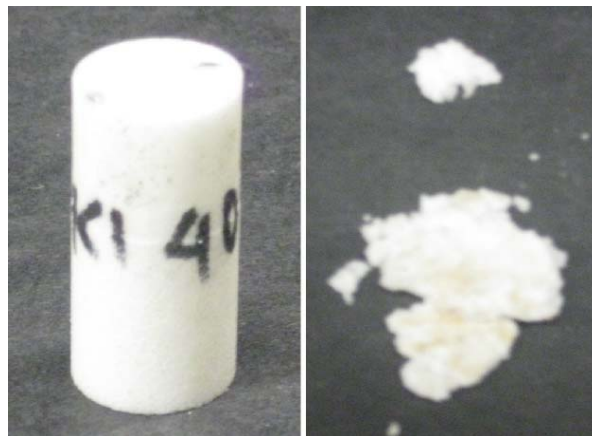
Figure 41. Impacted specimen of K1-40 syntactic foam
