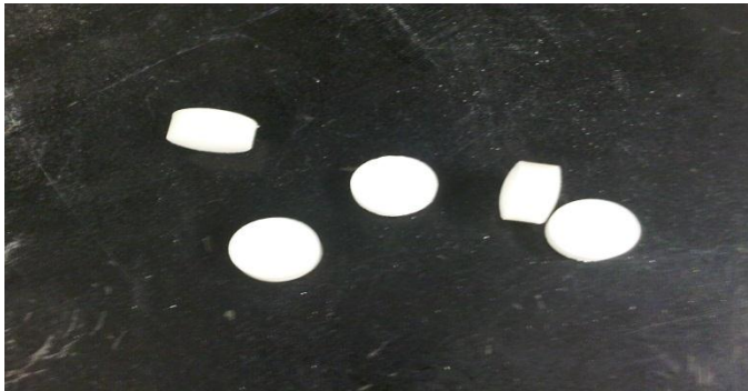
Figure 40: Tablets of HME mixtures containing 2% resveratrol by weight and Soluplus®.
