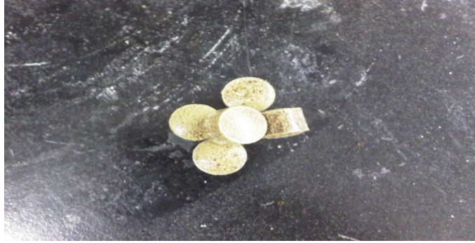
Figure 41: Tablets of HME mixtures containing 5% quercetin by weight and Soluplus®.
