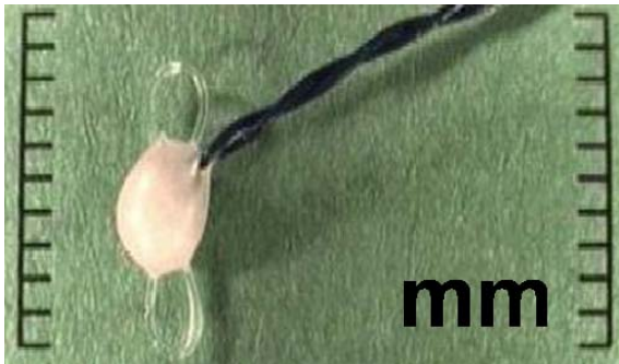
Fig 2. 2 mm sonometric crystal with suture loops.
