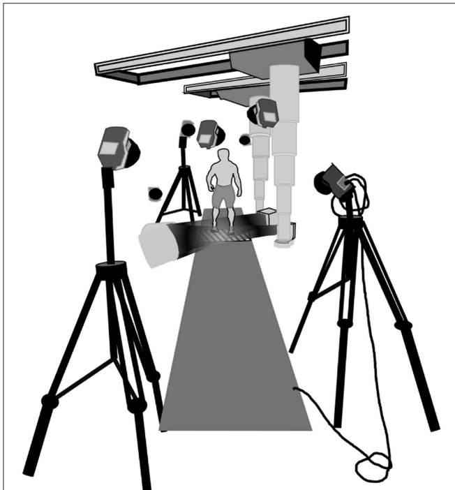
FIGURE 1 | Schematic depiction of the laboratory set up. The two x-ray sources were set at a 130° angle ipsilateral to each other. The intensifiers were stationed as close to the translucent Dragon Plate (AllRed and Associates, Elbridge, USA) as possible while maintaining visibility of the foot. The entire platform was evenly raised 0.60 m from the ground. Eight OMC cameras were stationed around the collection space to optimize viewing of the foot markers.
