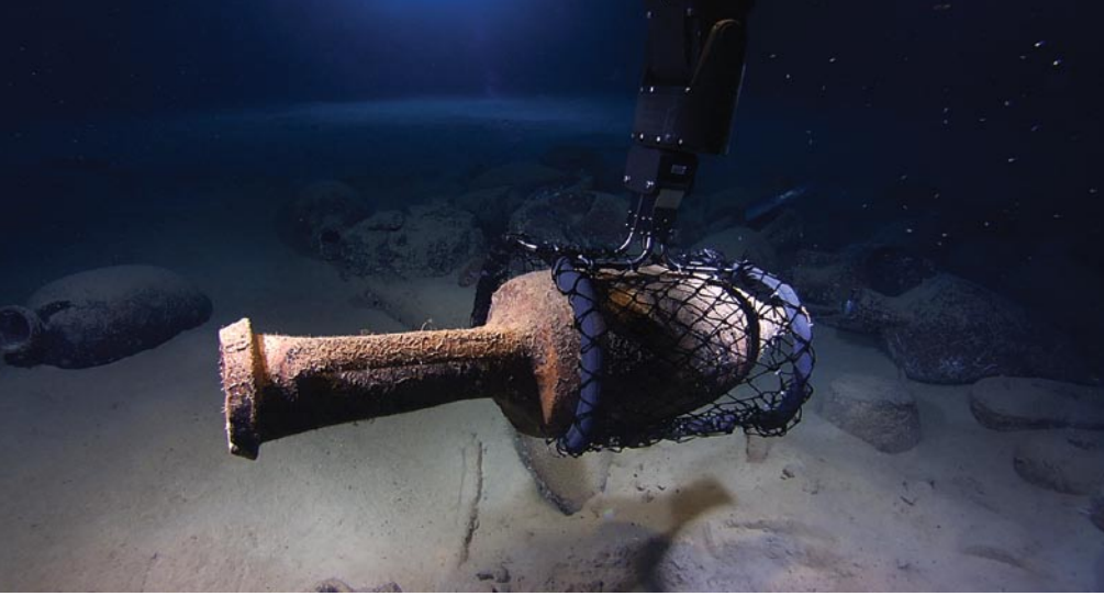
Figure 1. Hercules ROV grasping amphora from first century CE shipwreck at Skerki Bank.
