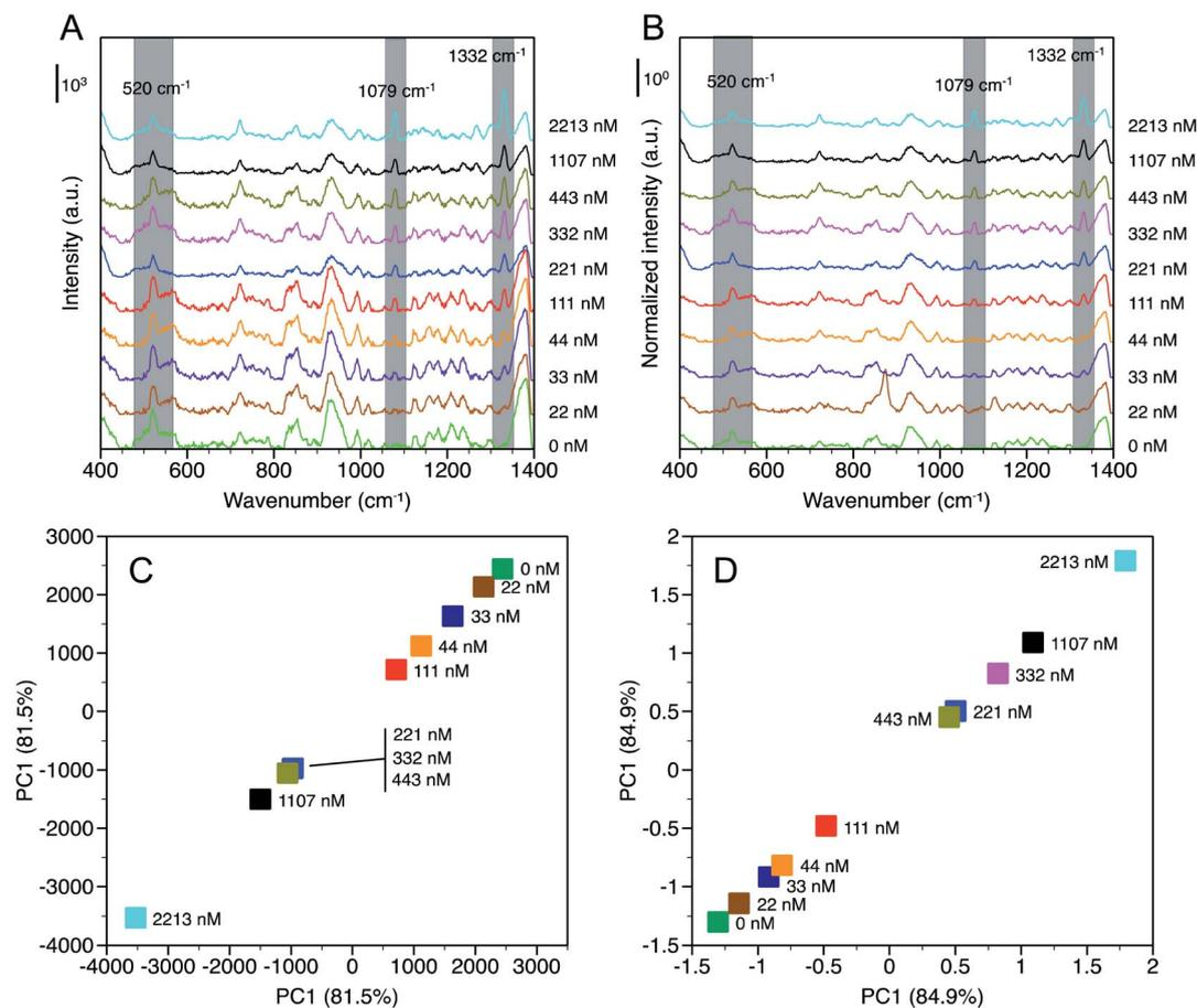
Fig. 3 SERS spectra of nitrate based on (A) intensity (baselined) and (B) normalized intensity (baselined + SNV). Greyed regions at  $1079\text{ cm}^{-1}$  and  $1332\text{ cm}^{-1}$  denote  $\text{NO}_3^-$  peaks used for adsorption analysis and the region at  $520\text{ cm}^{-1}$  denotes the silicon peak from the SERS substrate. PC1 plots corresponding for (C) baselined and (D) normalized time-averaged spectra over the range  $1000\text{ cm}^{-1}$  to  $1350\text{ cm}^{-1}$ .
