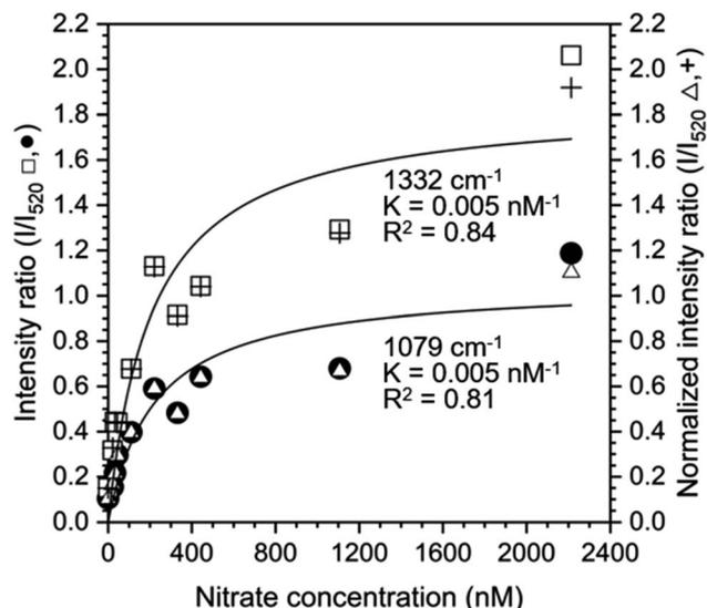
Fig. 5 Intensity and normalized intensity ratios ( $I/I_{520}$ ) based on the silicon peak at  $520\text{ cm}^{-1}$  and nitrate peaks at  $1079\text{ cm}^{-1}$  (closed circles ●, open triangles Δ) and  $1332\text{ cm}^{-1}$  (open squares □, plus signs +) as a function of nitrate concentration. The solid lines show the fitted Langmuir adsorption model and the Langmuir constant  $K$  and the goodness of fit,  $R^2$ , are reported.
