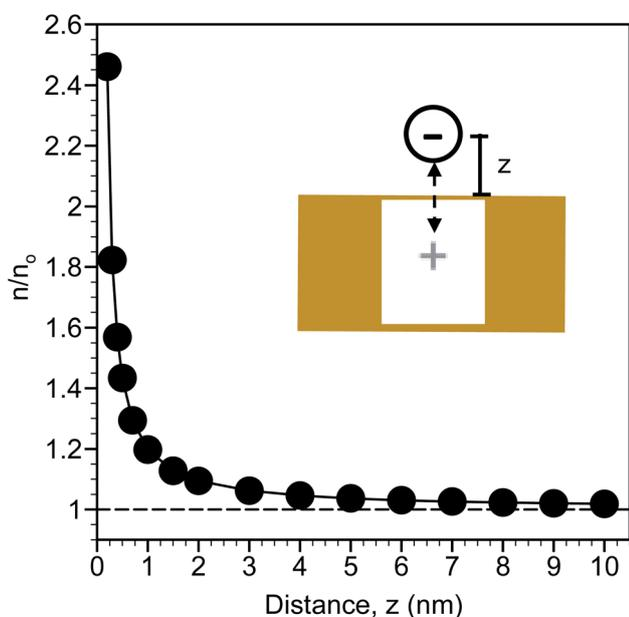
Fig. 2 Calculated monovalent ion distribution ( $n$ , normalized relative to the bulk concentration as  $n/n_o$ ) extending from a planar gold surface arising from "image charge", depicted in the schematic. The variable  $z$  represents the distance from the surface to the center of the ion.
