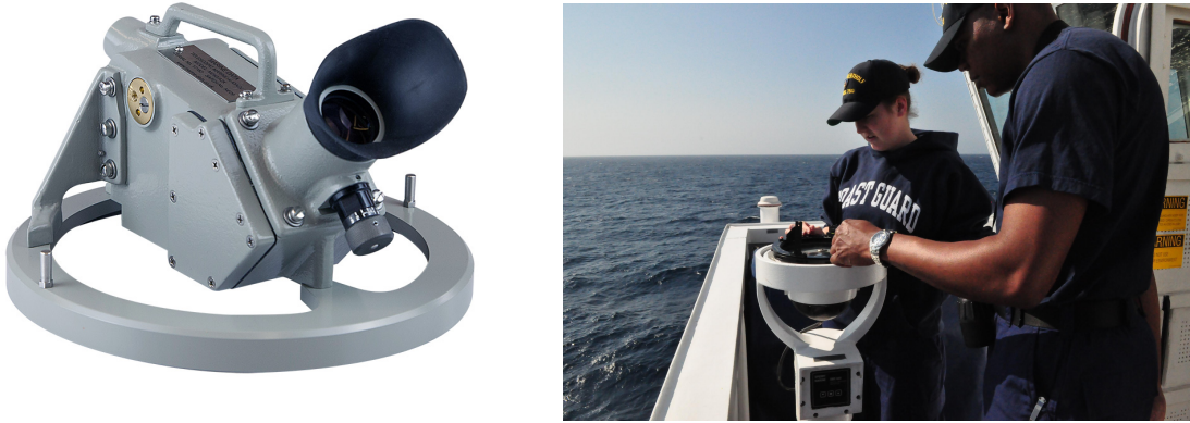
Figure 1: A typical alidade (left) and use of one on a Coast Guard vessel (right).
