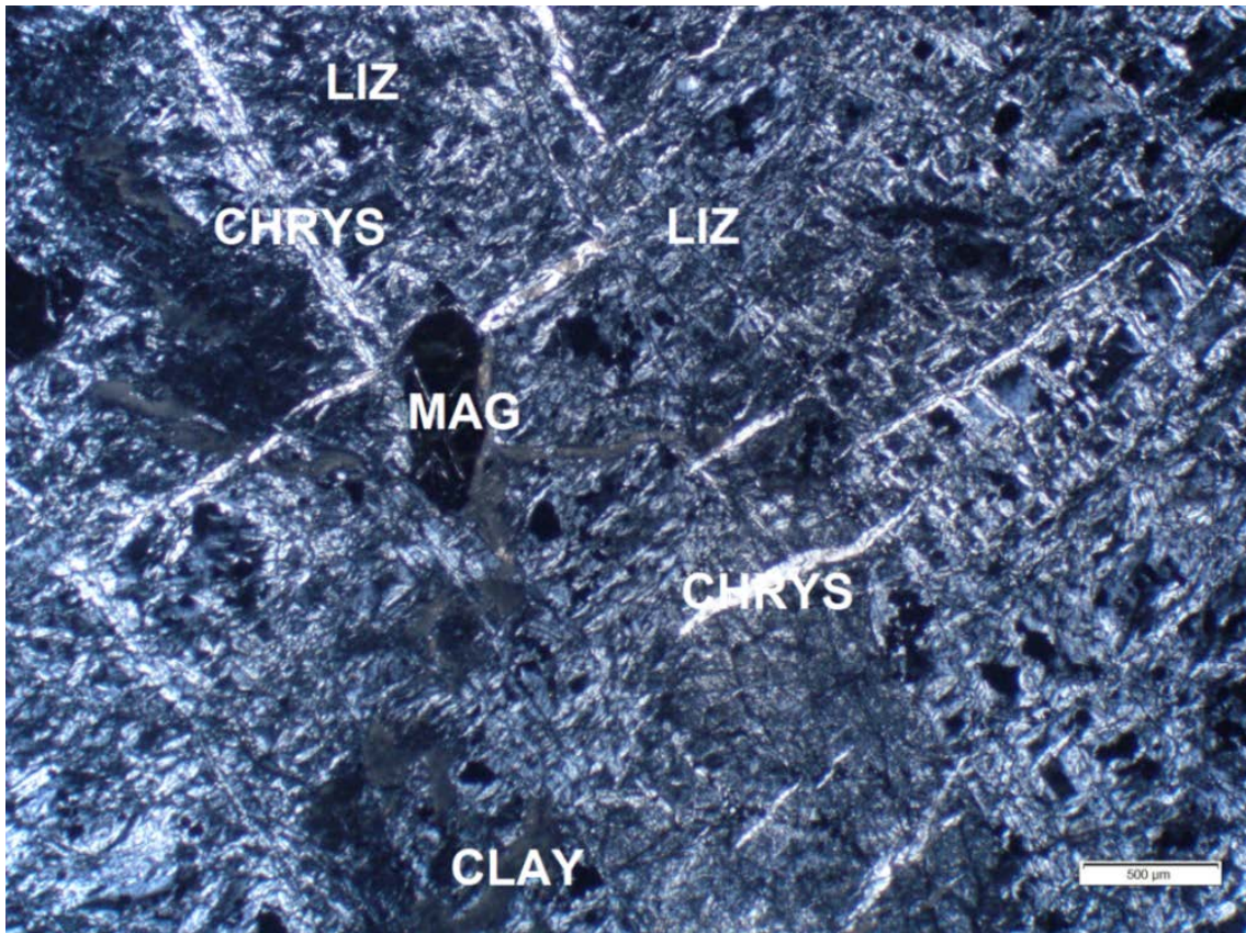
Fig. 27. 2x thin section from CROMO2-134 at 41.15 m depth. The thin section confirms the results from the XRD. Lizardite, the mesh-like white and blue matrix, makes up most of the slide, with white veinlets of chrysotile and scattered black blebs of magnetite. Some unidentifiable clay minerals are present as well as opaque brown steaks and smears.
