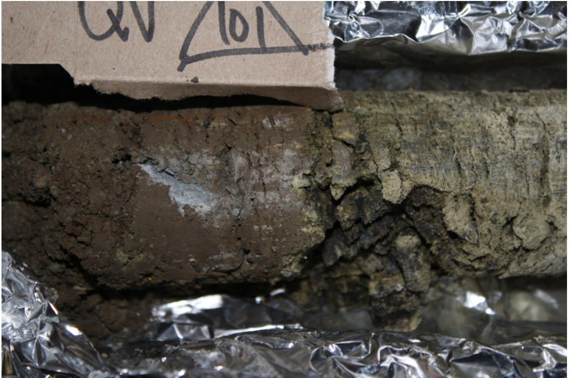
Fig. 18. Core taken from first 0.9 m of CROMO 2, essentially equivalent to serpentine-dominated valley topsoil. Photo credit: A. McCann.
