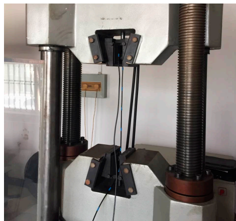
Figure 11. The experimental setup for the axially tensile strain test.
