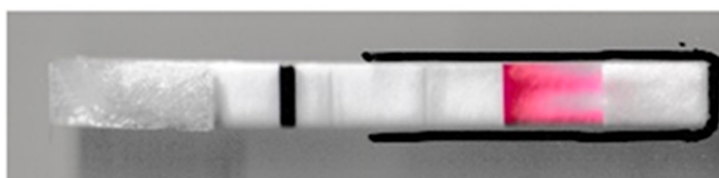
Figure 5. Lateral flow strip that was previously designed and tested. Color streaking and non-uniformity was observed in the detection zone.
