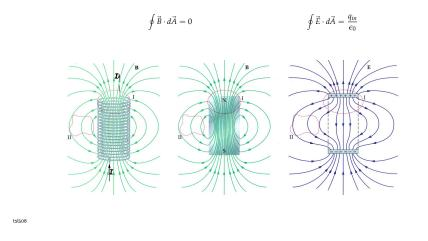
This slide shows two realizations of a magnetic dipole (left and center) and one realization of an electric dipole (right).
