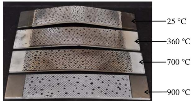
**Fig. 22** Post-mortem images of the specimens tested at 25 °C, 360 °C, 700 °C and 900 °C under blast loading.
