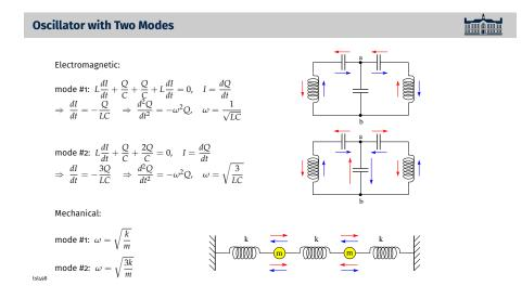
Here we return to an electromagnetic oscillator without damping and its mechanical analogue. The LC circuit with two inductors and three capacitors can oscillate in two different ways (named modes), depending on what the initial state is.
