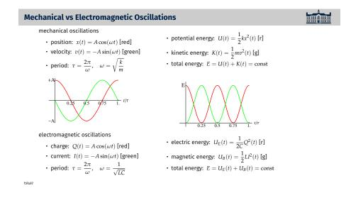
This slide emphasizes the correspondence between attributes of the mechanical oscillator on top and the electromagnetic oscillator at the bottom.
