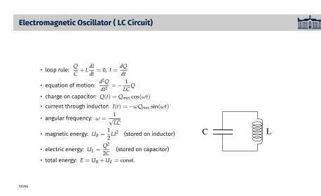
The *LC* circuit is an electromagnetic oscillator. We begin its analysis with the loop rule as usual [first item]. We recall that the current I(t) is the derivative of the charge Q(t) on the capacitor. This relationship is analogous to the velocity and position variables on the previous page.
