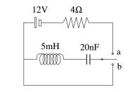
When the switch is closed to  $\mathbf{a}$  we have an *RLC* circuit including a battery. The loop rule includes four terms:
