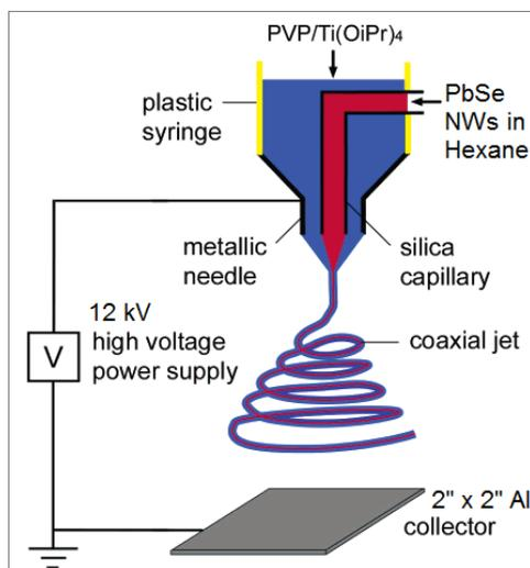
**Figure 4.** A schematic illustration of the co-axial spinneret, adapted with permission from [29]. Copyright 2004 American Chemical Society.
