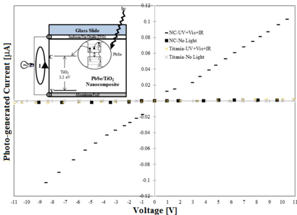
**Figure 3.** Current-Voltage ( $I-V$ ) curves for dark-current and photo-current testing of the electrospun nanocomposite compared to the neat electrospun  $\text{TiO}_2$  (inset: Schematic showing the energy band diagram for the nanocomposite and the flow of current through the fabricated testing device. This consists of the test material—either the neat anatase titania or the nanocomposite—sandwiched between aluminum foil and an ITO-coated glass slide).
