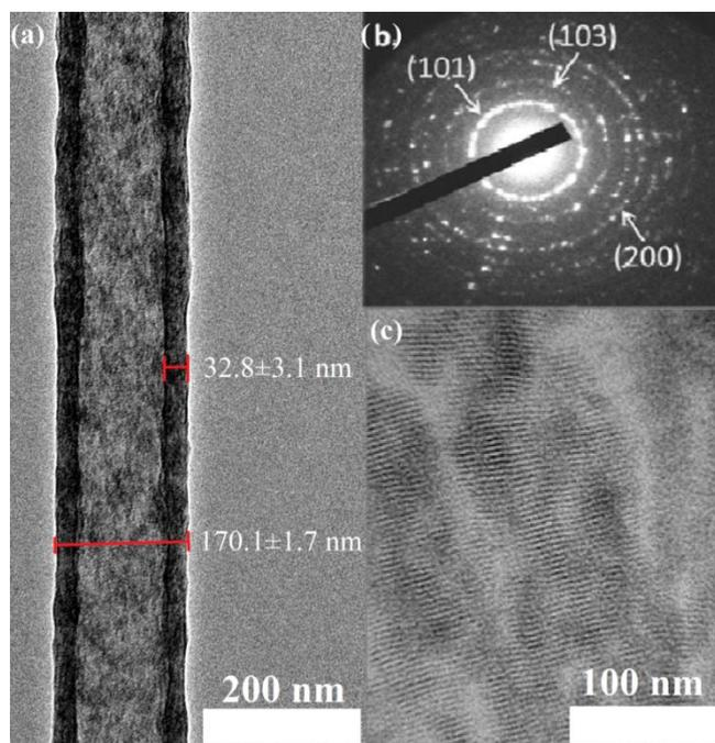
**Figure 1.** (a) TEM micrograph showing the high uniformity and reproducibility of the electrospun hollow  $\text{TiO}_2$  nanotube diameter and wall thickness, each with very small standard deviations; (b) Electron diffraction pattern indicating the presence of anatase  $\text{TiO}_2$ ; (c) TEM micrograph of the standalone  $\text{PbSe}$  nanostructures.
