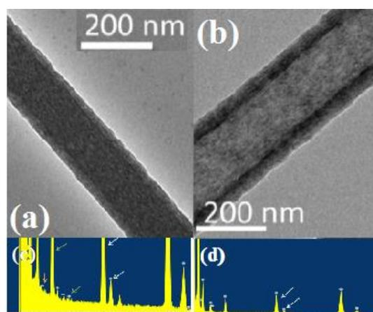
**Figure 2.** TEM micrographs of the  $\text{TiO}_2$  nanotubes (a) with and (b) without the PbSe nanostructures, illustrating that the PbSe nanostructures can be implemented into the  $\text{TiO}_2$  nanotubes without changing the overall nanocomposite morphology. EDX analysis of the  $\text{TiO}_2$  nanotubes (c) with and (d) without the PbSe nanostructures, showing (in (c)) an equal ratio of Pb and Se and the presence of the PbSe nanostructures.
