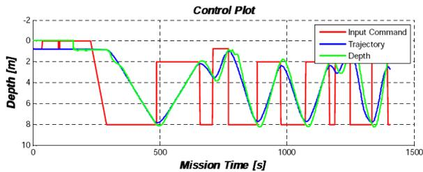
Fig. 9. Test of the profile behavior at 2.5m/min, 5m/min and 10m/min rates. Note the rate changes were not made to coincide with the end of a complete cycle.
