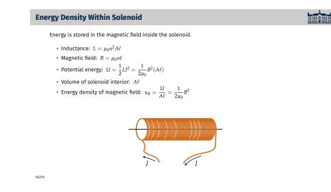
We use the solenoid design for a demonstration that the energy stored on the inductor is located in the magnetic field B.
