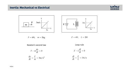
This page is intended to portray the aspect of inertia associated with a current flowing through an inductor using a mechanical analogy.
