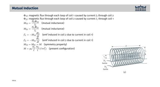
Mutual inductance, as opposed to self induction, covers an important set of applications of Faraday's law. The slide shows a setup with two coaxial solenoids, for which the effect is easily demonstrated.
