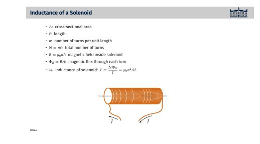
Here we calculate the inductance L of a solenoid with given specifications as stated in the first three items. The fourth item combines the previous two for use in the definition of inductance.
