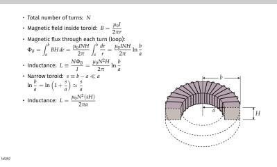
We have discussed earlier that when we bend a solenoid into the shape of a doughnut we get a toroid. In the toroid shown, the turns of wire are rectangular, which simplifies the calculation of L a bit.
