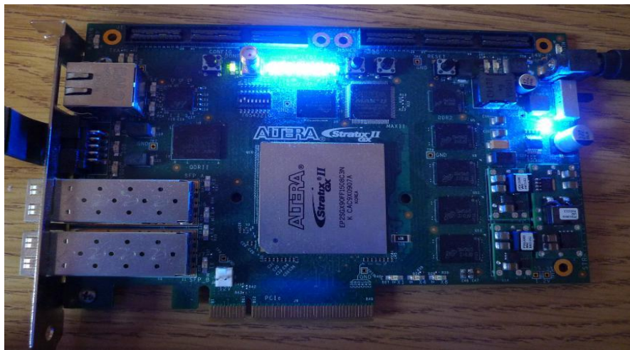
Figure 2.6. The prototype board based on Altera Stratix II GX EP2SGX90 PCI Express platform.
