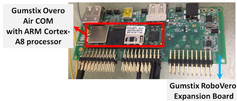
Figure 5.3. The prototype based on Gumstix Overo Air COM and RoboVero expansion board.
