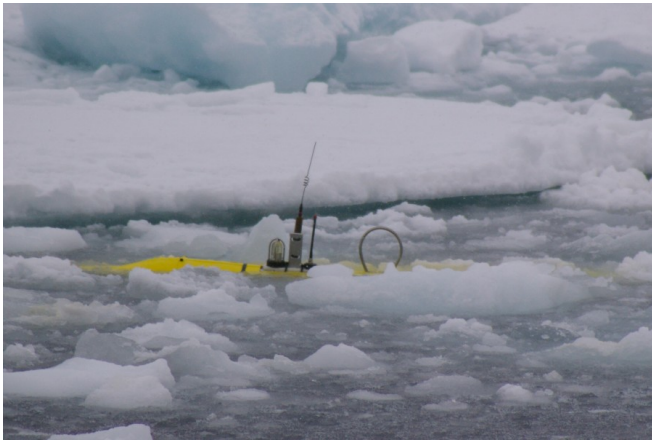
Fig. 8. Puma surfaces in ice near the pond edge after PUMA0001.
