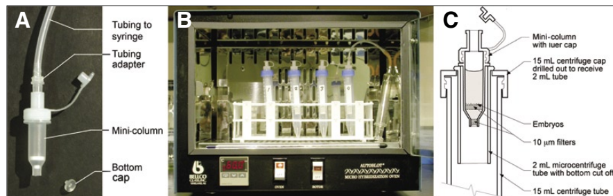
Figure 1. Mini-column apparatus for whole-mount in situ hybridization. (A) Mobicol mini-column set up for the WMISH procedure. (B) Four columns set up for use in the hybridization oven. Mobicols are inserted in open-bottom 2 mL microcentrifuge tubes inserted through holes in the tops of 15 mL centrifuge tubes. (C) Cross-section diagram of the mini-column apparatus.
