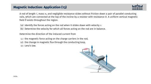
(a) There are three forces acting on the rod: (i) the weight  $\vec{w} = m\vec{g}$  pointing vertically down, a normal force  $\vec{N}$  perpendicular to the plane of the rails toward the upper right, and a magnetic force  $\vec{F} = I\vec{l} \times \vec{B}$  in the plane of the rails toward the upper left.
