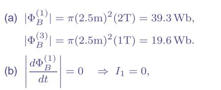
$$\left| \frac{d\Phi_B^{(3)}}{dt} \right| = |\pi(2.5\text{m})^2(-1\text{T/s})| = 19.6\text{V}$$
