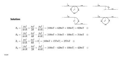
From earlier we know that a thin wire bent into a circle of radius R generates a magnetic field  $B_{\circ}$  at its center and a very long, thin straight wire generates a magnetic field  $B_{|}$  a distance r from it if the wires carry a current I:
