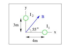
Here is the reverse of the application from the previous page. The orientation of the two wires and their positions in the xy-plane are the same. However, we do not know the two currents  $I_1$  and  $I_2$ , not even if they are directed in  $(\odot)$  or out  $(\otimes)$ .
