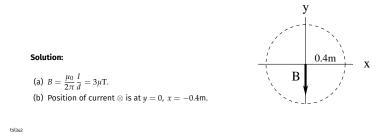
This is an even simpler application of a long, thin, and straight wire carrying a current.
