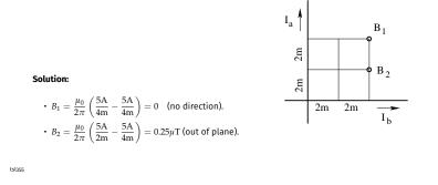
In this application, we have two very long wires, perpendicular to each other and positioned in the plane of the paper as shown. Both wires carry a current of 5A in the directions shown.
