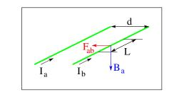
Next we consider two very long, thin, parallel, conducting rods, a distance d apart, both carrying currents. The currents  $I_a$  and  $I_b$  flow in the same direction, which causes the rods to experience an attractive interaction force.
