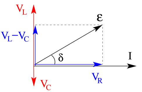
Relation between  $\mathcal{E}_{max}$  and  $I_{max}$  from geometry:
