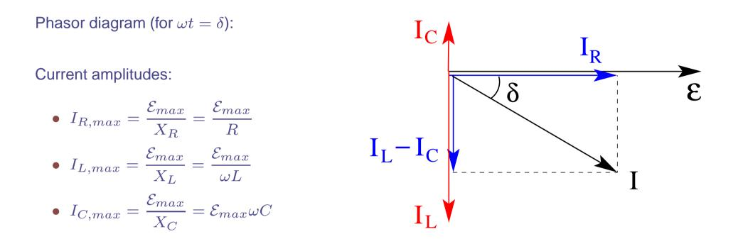
Relation between  $\mathcal{E}_{max}$  and  $I_{max}$  from geometry:
