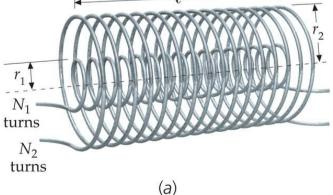
Establishing a current in the inductor requires work. The work done is equal to the potential energy stored in the inductor.
