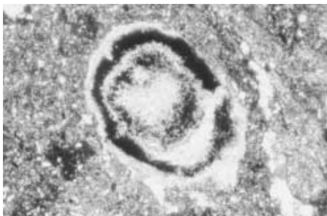
FIGURE 4 —Photomicrograph of concentric rings of ferruginous oxides inside a carbonate nodule at Ghost Ranch. Picture taken under crossed-polars; field of view is 1.3 mm wide.
