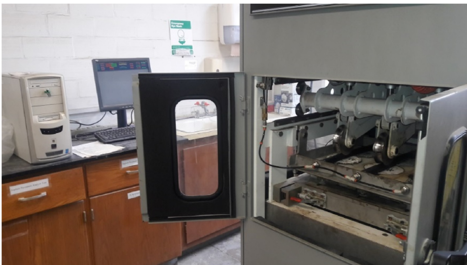
Fig. 4. Installed specimens on Asphalt Paving Analyzer (APA) machine.
