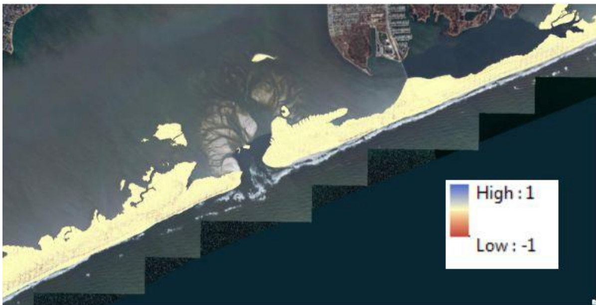
Fig. 8. Differences between DEMs used by each Study in FIIS. Blue represents greater elevation heights of the DEM used by the Sandy Study to the DEM used by the Servicewide Study (similarly represented by red).
