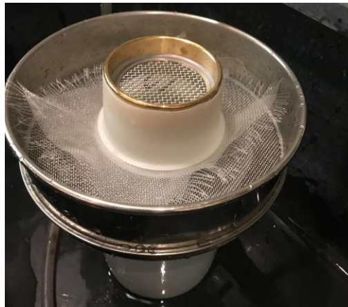
Figure 6: Wet sieving set up. A 2-mm sieve on top of a 1-mm sieve.
