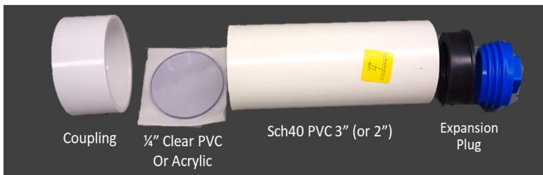
Figure 1. Housing is a standard-sized (3-inch PVC) or Mini-sized (2-inch PVC).
