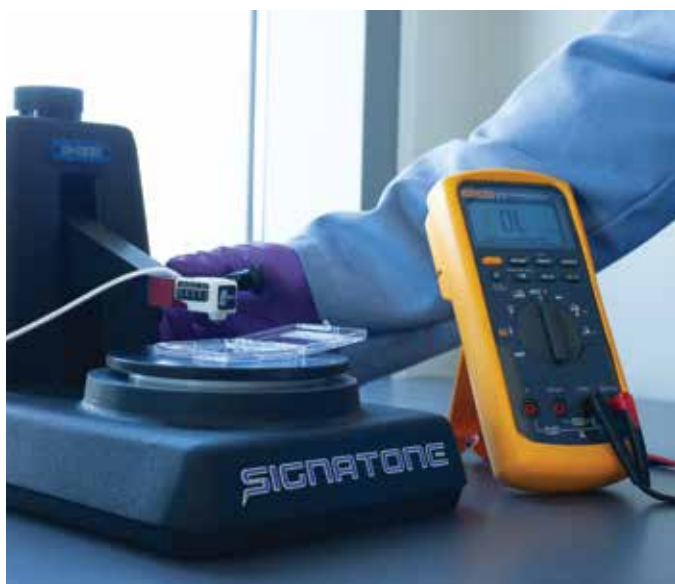
This is a thin film conductivity measurement system. When designing nanofabricated electronic sensors it is helpful to be able to independently characterize their properties.
