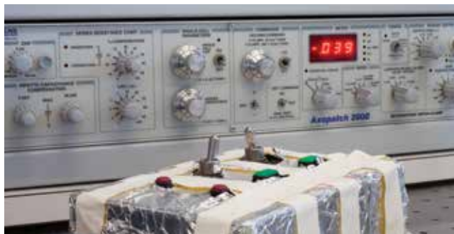
Benchtop control electronics for sensing single molecules using nanopores.
