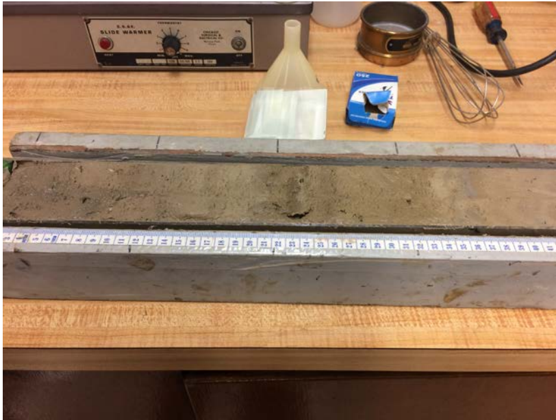
Figure 5: Opened core. Ruler alongside the core indicates cm below top of the core.
