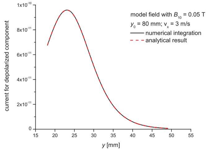
FIG. 6. (Color online) Depolarization current for downward motion in the magnetic field for parameters  $y_0 = 8$  cm,  $B_{10} = 0.05$  T, and  $v_x = 3$  m/s. Direct numerical integration, represented by the solid curve, coincides with the analytic result shown by the dashed curve, with a maximum deviation of 1% over the entire range from upper to lower turning point ( $y_u = 49.56$  mm,  $y_l = 18.08$  mm).
