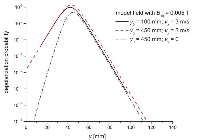
FIG. 2. (Color online) Depolarization probability, given by Eq. (34) multiplied by  $m/\hbar$ , as a function of neutron position for drop heights  $y_0 = 450$  mm and 100 mm, stabilization field parameter  $B_{10} = 0.005$  T, and neutron velocity component  $v_x = 3$  m/s or zero. The sharp peak occurs in the region where the gradient of field angle  $\theta$  is largest.
