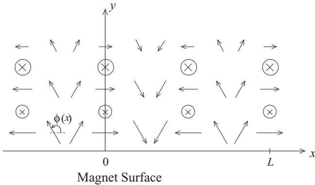
FIG. 1. For our field model, the arrows show the Halbach magnetic field  $\mathbf{B}_H$  as it rotates in the  $(xy)$  plane. Its magnitude  $B_H$  decreases exponentially with height  $y$  and is represented by the arrow length using a log scale. The angle  $\phi = -Kx$  of the Halbach field is also shown. The superimposed stabilization field  $\mathbf{B}_1$  in the  $z$  direction increases slowly with  $y$  as in Ref. [14] and is symbolized by the crosses of variable size.
