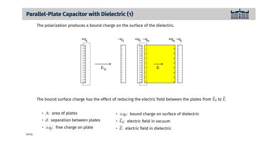
On the slide we see the same charged parallel-plate capacitor without dielectric (left) and with dielectric (right). All relevant specifications are listed.
