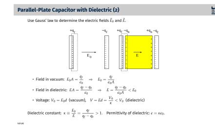
The electric field  $E_0$  between the plates in the absence of a dielectric can be inferred from Gauss's law in the form of a pizza box (shown dashed in cross section) that envelops the inside surface of the plate with  $+q_f$  on it. The result is shown as the first item on the slide.
