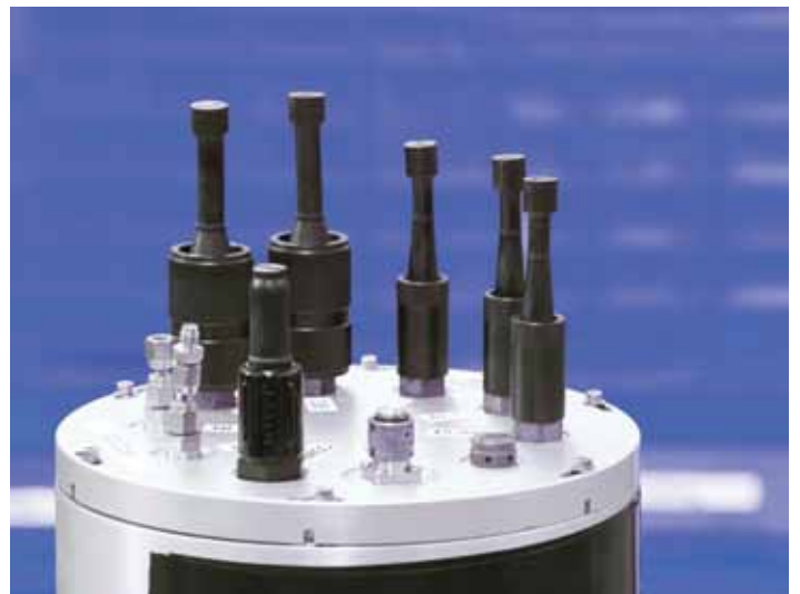
Underwater mass spectrometer used to measure water properties in the freezing ocean.
