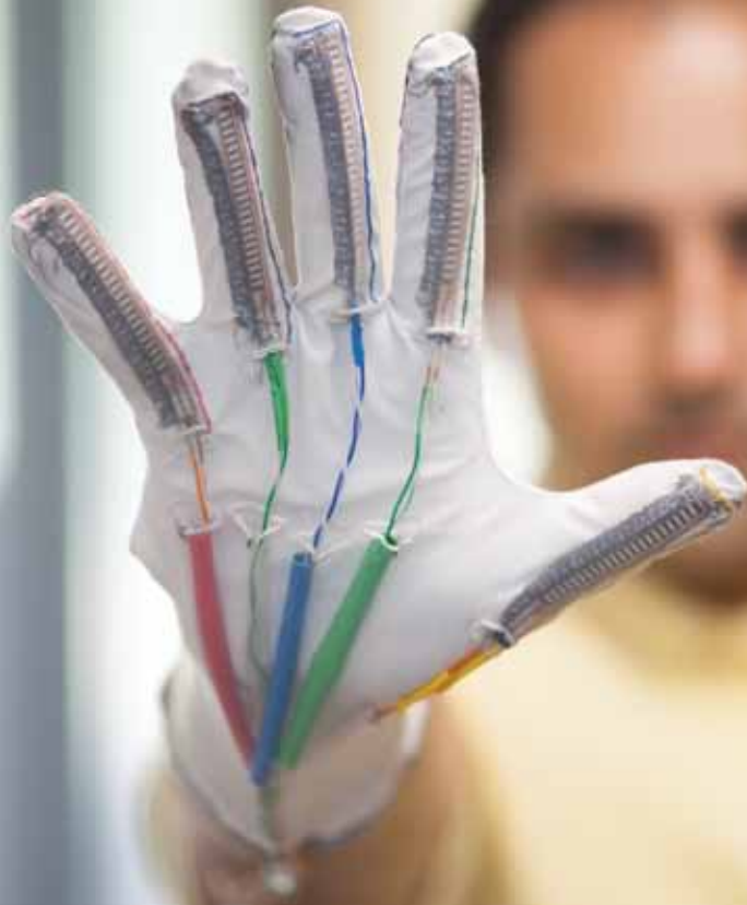
Smart Glove which can measure tremors and movement difficulties in Parkinson's disease patients. These gloves are woven with high-resolution motion and stretch sensors connected to an on-board computer with wireless connectivity.
