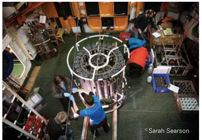
Water sampling for ocean properties using a 24 bottle CTD rosette.
