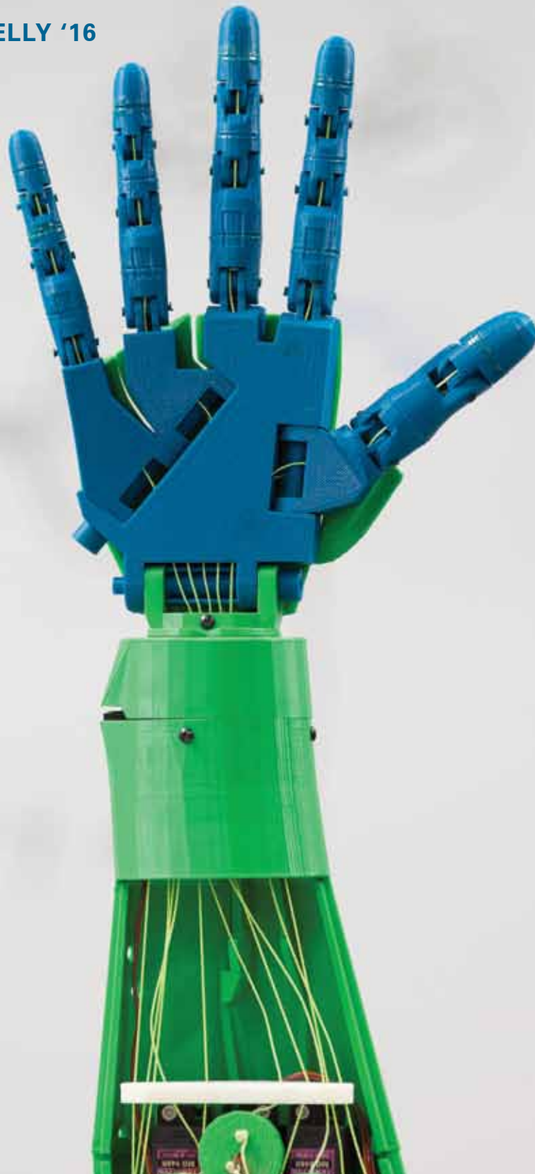
3D-Printed Robotized Hand, developed to help amputees.
