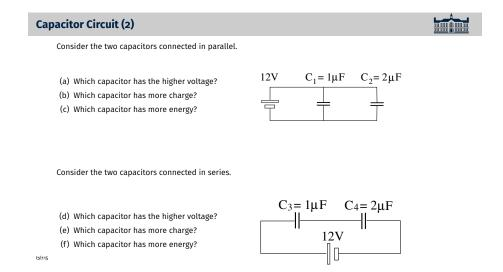
Here we introduce a new device, the voltage source or battery, represented by two parallel rectangles. The tall and thin rectangle is at higher potential than the short and wide rectangle. The potential difference is the voltage Vsupplied by the battery to the circuit, here 12V.
