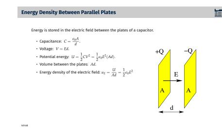
We use the parallel-plate geometry to determine the energy content of an electric field. Our choice is motivated by the uniformity of the electric field E in the space of volume Ad between the plates, where A is the area of each plate and d the distance between them.
