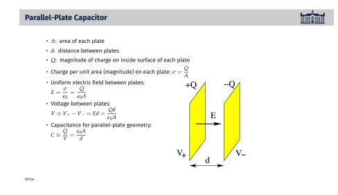
For some capacitor designs, it is simple enough to determine the capacitance in terms of the geometric specifications.
