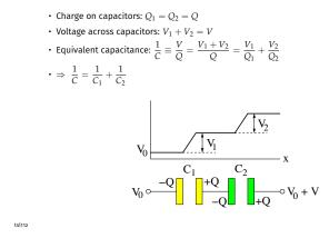
A series connection of two capacitors consists of three conductors, one on the left at potential  $V_0$ , one on the right at potential  $V_0 + V$ , and one in the middle at a potential to be determined.
