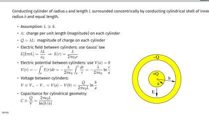
A different design uses coaxial cylinders as shown here in cross section. The capacitance does not depend on which conductor is charged positively. However, a choice has been made for the calculation of C.
