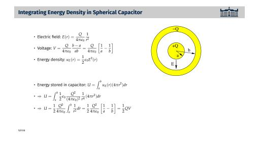
If the energy-density expression derived on the previous page is indeed general, then we can use it to determine the energy stored in a capacitor where the field is not uniform.
