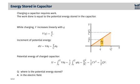
Placing a charge Q on a capacitor, i.e. charge +Q on one conductor and charge -Q on the other, is like lifting a weight or compressing a spring. The process requires work.
