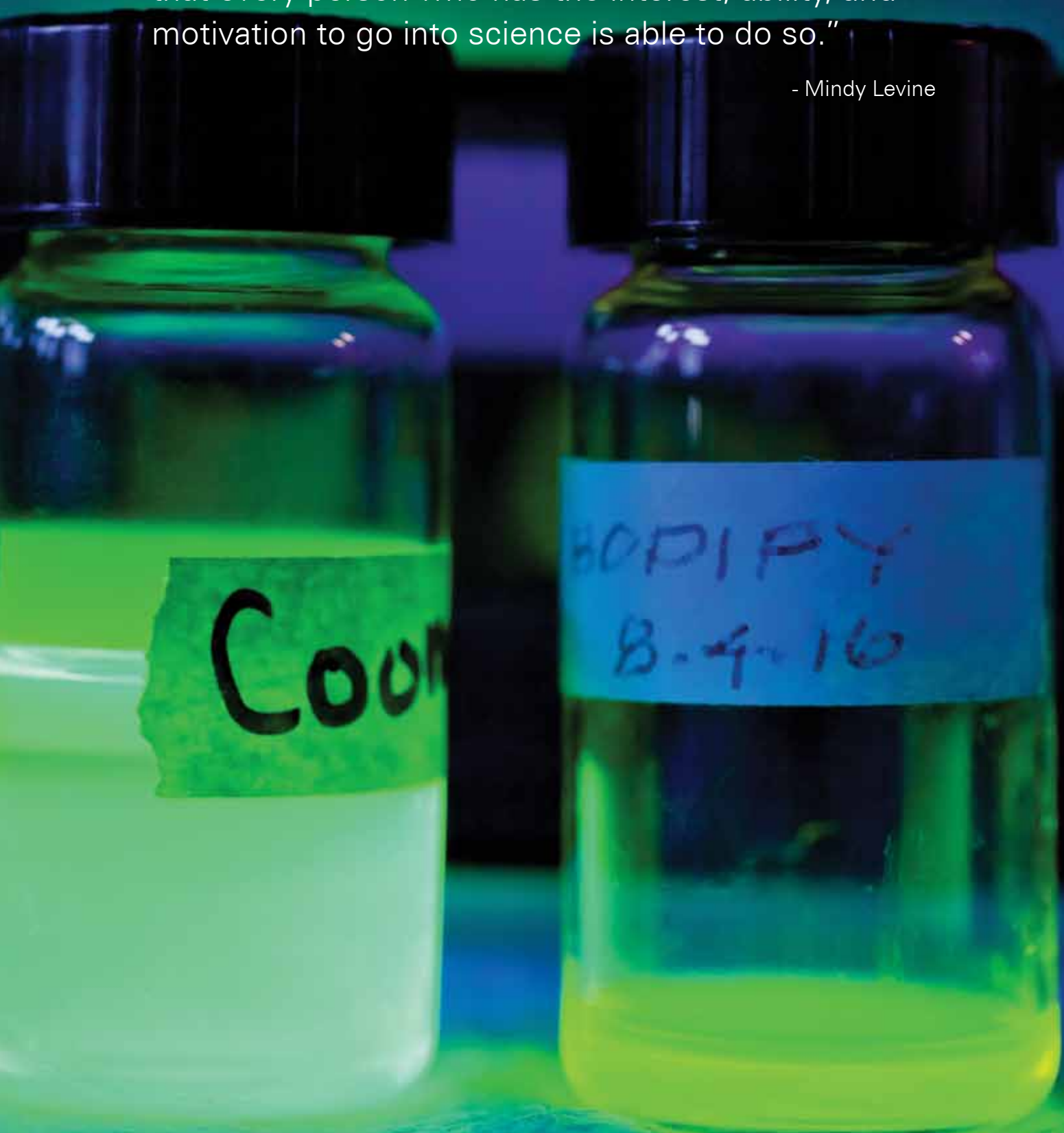
Fluorescence indicators that change color in the presence of the toxic chemicals.
