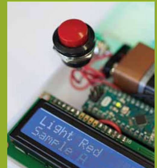
3D-printed handheld device for monitoring the harmful algal blooms.
